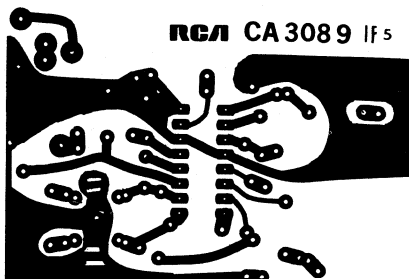
a) Bottom view of printed-circuit board.
